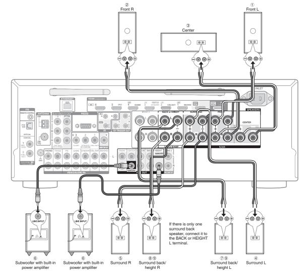
**Important:** Connect speakers with 6  $\Omega$  to 16  $\Omega$  impedance. Using a speaker with less impedance than the supported value may result in failure. (\*)
